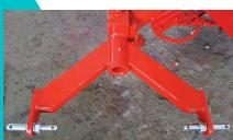
Articulated drawbar with 2 points for tractor attachment. Ease of entry and exit from rows, in less space. It has 2 pins to connect to the tractor's 2 points linkage.
