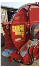
Window opening under the turbine to allow unloading at the centre of the track, under the trailer. The spreader is equipped with a hydraulic side door (by means of a cylinder placed on the front of the trailer) that closes the side exhaust, and opens the central exhaust under the trailer.
