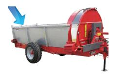
Hot galvanized side walls. On request is also possi-ble to galvanize the complete frame.
