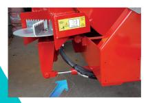
Hydraulic inclination of the lateral disc. It allows to adjust the inclination of the disc by a hydraulic cylin-der, by tractor oil distributor.
