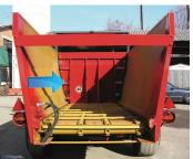
Rear door automatically advancing together with con-veyor chains, to push manure to the turbine with end stroke valve.
