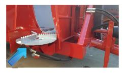
Lateral disc, driven by hydraulic motor. On request, for use in vineyard and orchard to localize the manure on a row. It can be manually tilted to obtain a better localiza-tion (longer or shorter spread)
