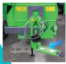
Articulated drawbar with mechanical lock. Ease of entry and exit fron rows in less space (follows the tractor track) It has 2 confi gurations: locked with pin (use on the road), unlocked/articulated for use on row. Check compatibility of the drawbar with tracotr towing bar.
