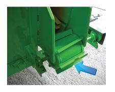
Side roller STANDARD device: shaft with rotor or blade, depending on model, for lateral distribution. Standard device on all model with turbine system. It prevents the fall of manure in the area of passage of the tyre.
