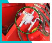
For localizer plate: flow control to adjust the rotation speed of the tray
