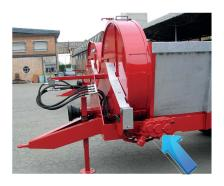
Hydraulic chain conveyor with gearbox adjustable speed with orbital motor + shock valve and flow regulator to adjust the speed of the conveyor chains
